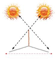
Find a sunny area on the ground. Avoid using this method in the middle of the day. During noon, the shadow will shrink and almost disappear because of the high position of the sun. This will not be optimum to give you an accurate East-West line.
